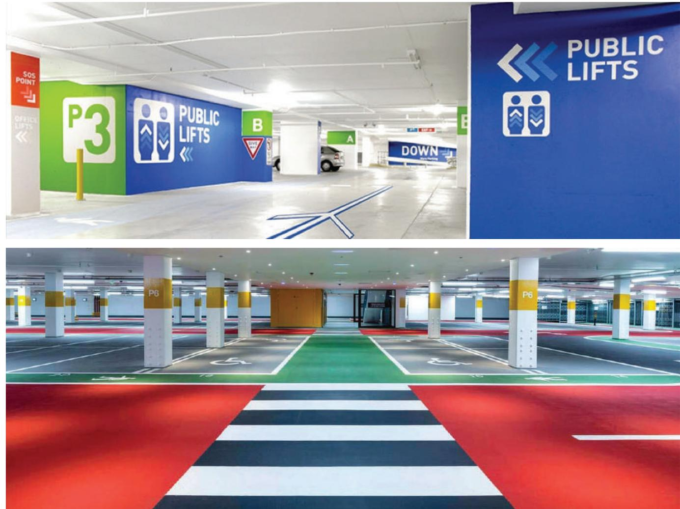
**Figure 1 & 2:** Use of clear delineation of car and pedestrian areas with strong wayfinding elements make navigating car park buildings safer for all users
