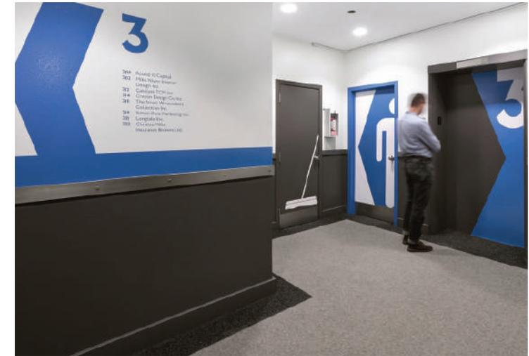
**Figure 1:** There is a clear and unobstructed area outside of the lift in this otherwise busy lobby that is serving a WC, storage cupboard and lift. The floor of this office is subdued and a single consistent colour to avoid confusion with the wayfinding elements of this lift lobby.
